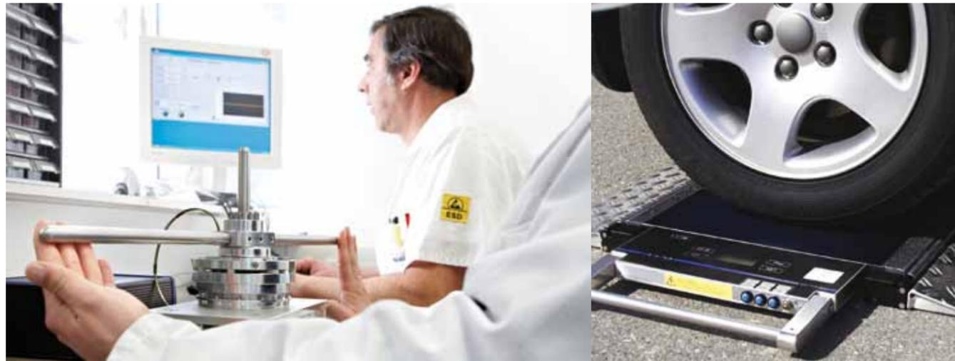
Force measurement offers many application possibilities. That is why we develop individual force gauges and systems for various fields of application that consist of our force transducers and displays which satisfy all customer requirements. Examples of use can be found in motor vehicle test engineering, overload detection for building cranes and rope winches as well as in monitoring press-fit procedures.
